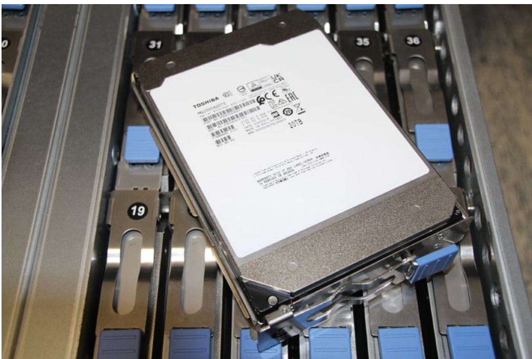
Picture 5: Toshiba MG10SCA20TE HDD in Promise tray
