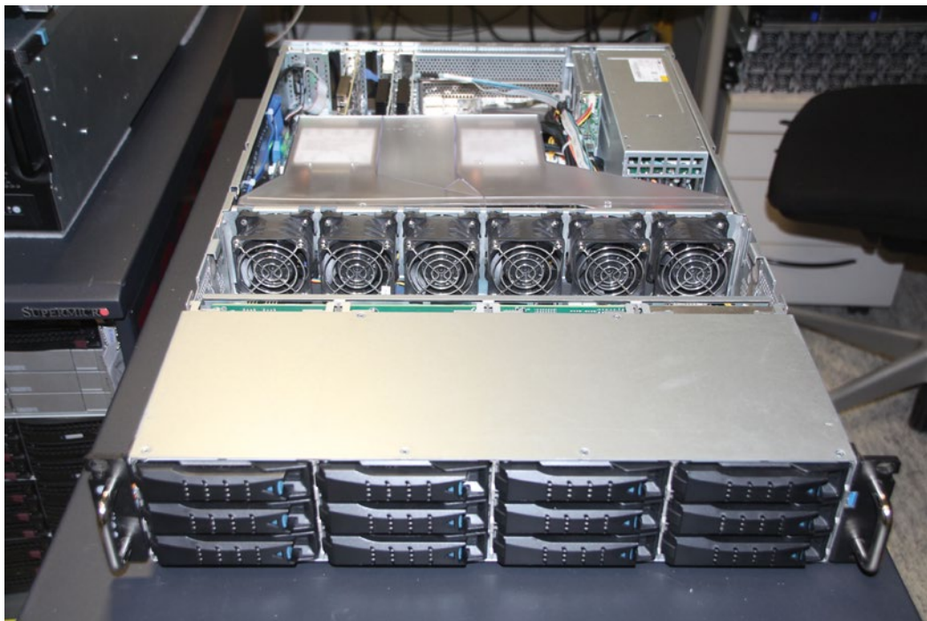
Picture 2: SB202-TU head node server from AIC
