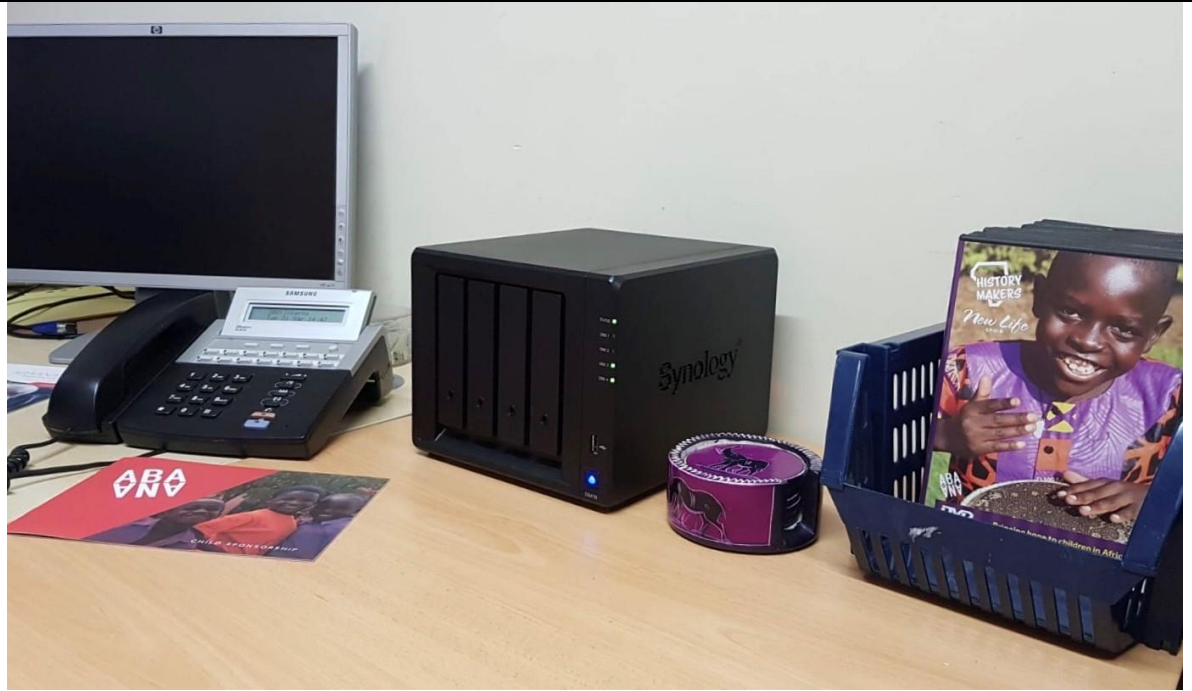
Figure 1 – The new RAID storage, featuring four 4 TB N300 NAS HDDs from Toshiba, takes pride of place in the Abaana charity's office.
