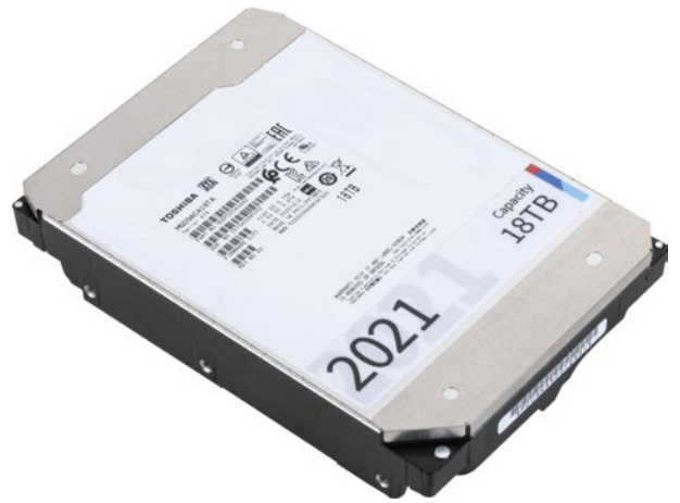
Figure 8: In 2021, a new generation of hard disk drives entered the scene, relying on the new MAMR (microwave-assisted magnetic recording) method. The first model had a capacity of 18 Terabytes, and its successor in 2022 has already brought it to 20 Terabytes. (Source: Toshiba Electronics Europe)
