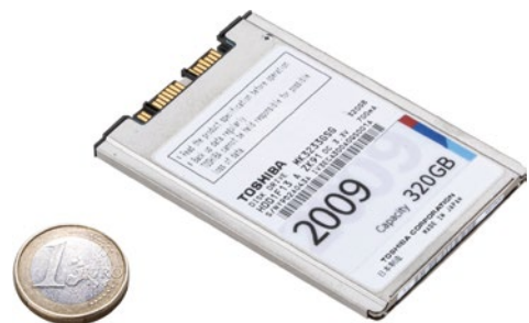
Figure 6: This flat 1.8-inch hard drive from 2009 is equipped with a single magnetic disk that can store 320 Gigabytes and is used in compact notebooks, among other things. (Source: Toshiba Electronics Europe)
