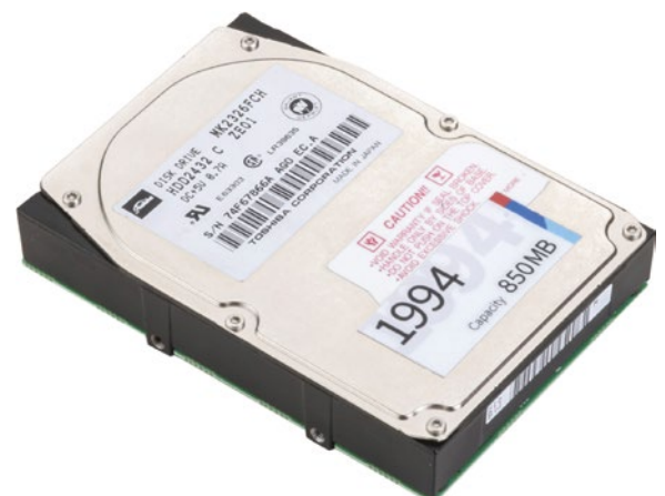
Figure 2: At the end of the 1980s, 3.5-inch drives became popular; here is a model from 1994 with 850 Megabytes. The form factor is still standard in PCs, servers and storage systems today. (Source: Toshiba Electronics Europe)
