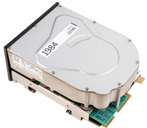
Figure 1: A hard disk model from 1984 that stores 20 Megabytes. At that time, the drives were increasingly being installed in PCs, but at 5.25 inches they were still much larger than today's hard disks. The interfaces were also not yet standardised – PATA came later. (Source: Toshiba Electronics Europe)
