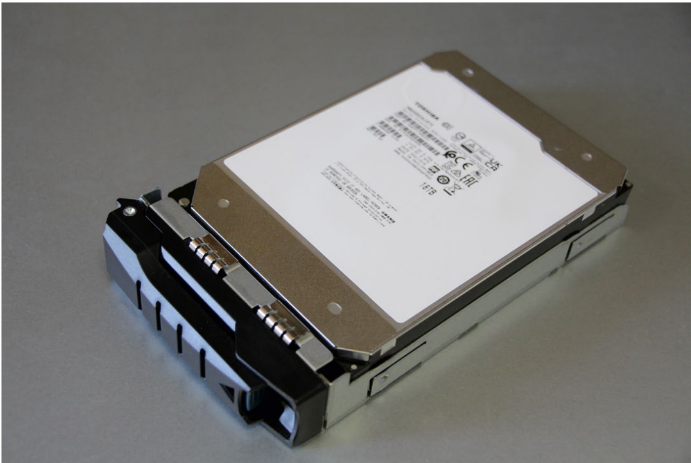
Picture 2: Toshiba HDD MG09SCA18TE in JBOD tray.
