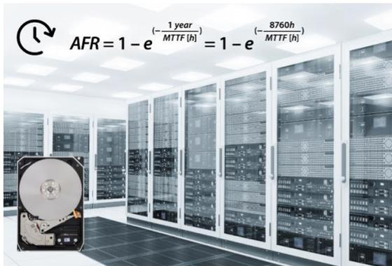
There is still no way around HDDs for the cost-effective provision of storage capacity. Different applications require the use of different HDDs. The decisive selection criteria are reliability and operating conditions.
